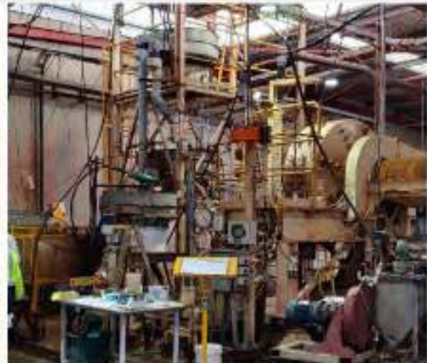
Pilot SAG and Ball mill to grind Longonjo ore for flotation
