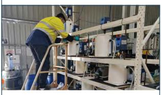
Carbonate product precipitation circuit setup
